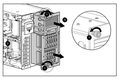
Figure 2-18. Removing the Ultra2 hot-plug drive cage assembly
